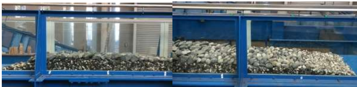
(b) Gravel mount with averaged size 16.5 mm (inside region), crash stones of averaged size 92.1 mm (upstream installation part) and cobble stones of averaged size 47.5 mm (downstream installation area)
