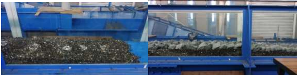
(a) Gravel mount with averaged size 5.3 mm (inside region), crash stones of averaged size 92.1 mm (upstream installation part) and cobble stones of averaged size 47.5 mm (downstream installation area)
