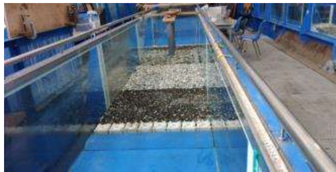
Figure 46. Installation of assembled boulders, crashed stones, and pebbles stones
