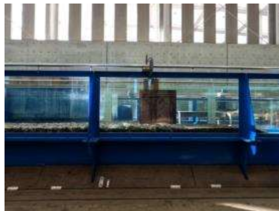
Figure 48. Installation of consecutively assembled boulders around long ellipse pier
