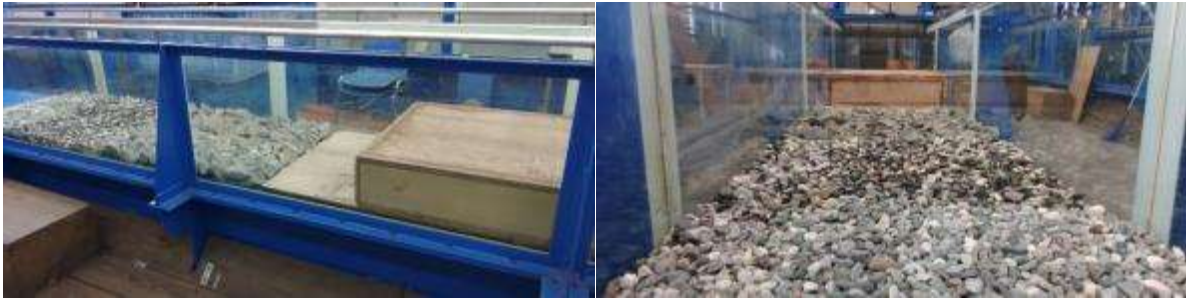
Figure 15. Physical model for both low drop structure and protection region due to assembled boulders
