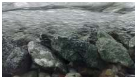
(c) Aerated flow above the assembled boulders
