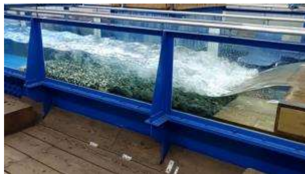
Figure 17. Flow condition downstream of low drop structure
