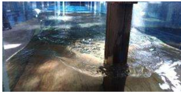
Figure 5. Deflected flows downstream of support pier
