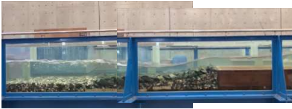
Figure 26. Flow condition at ramp with assembled boulders
