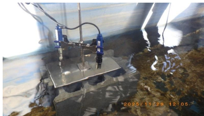
Photo 3. Installation position for pH and DO measurements in sharp-edged weir
