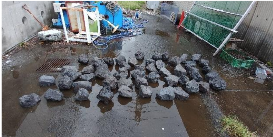
Photo 1. Oxidized Slag Boulders (tested 52 boulders)
