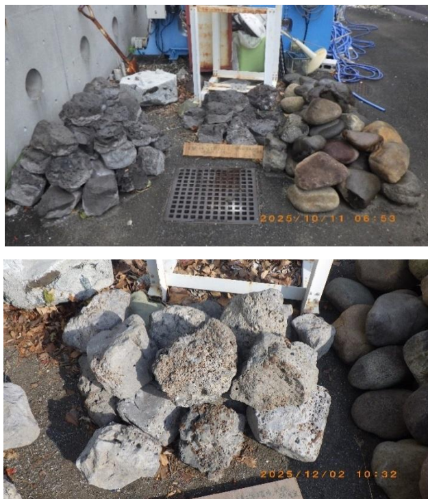
Photo 6. Condition of the oxidized slags one month after the first experiment in September
